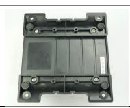
Remove the four mounting screws from the underside of the unit.
