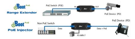
The Injector function requires the use of external power supply model PS-WRI-7.
